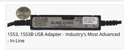
The product embeds the industry leading MIL-STD-1553 protocol engine AltaCore™ technology directly into the 1553-USB cable assembly. With this new product, a customer has all the advanced 1553 BC, RT and BM controls of card-board-based products via USB connection. With PCMCIA, PCCARD and Express Card interfaces being phased out of portable computers, Alta's
