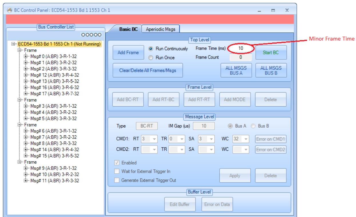
Therefore, the 100Hz messages occur 4 times in the major frame (every minor frame), the 50Hz messages occur 2 times in the major frame (every other minor frame), and the 25Hz messages occur 1 time in the major frame. Note that each of these occurrences of a given message has its own data buffer for receive messages – if you change the data you need to make the change on all occurrences of the message.
