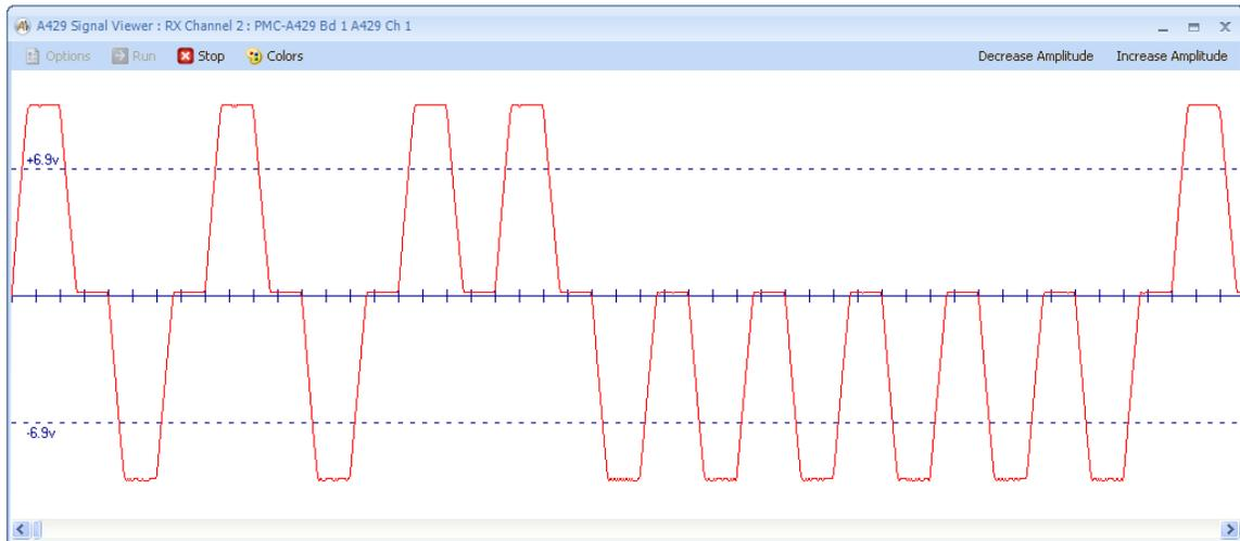
This shows a low-speed (12.5 KHz bit-rate) A429 signal.
