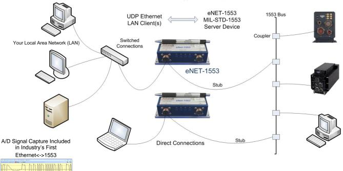
**eNet-1553**™ is an innovative product that provides "remoting" of 1553 operations on 10/100/1000 Ethernet IP/UDP local area networks (LAN). eNet-1553 is a small, low-power, rugged device that provides connectivity for one dual redundant 1553 bus and is ideal for remoting 1553 connections for in-field applications or point-point lab usage.
