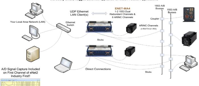
**eNet-MA4**<sup>™</sup> is an innovative product for "remoting" 1553 & ARINC-429/717 operations on 10/100/1000 Ethernet local area networks (LAN). eNet-MA4 is a very small, low-power, rugged device that provides real-time UDP connectivity to for 1-2 dual redundant 1553 (A/B) busses and 8 ARINC channels.
