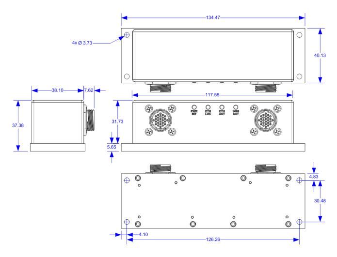
Figure 2. eNet-MA4 Dimensions (mm)
