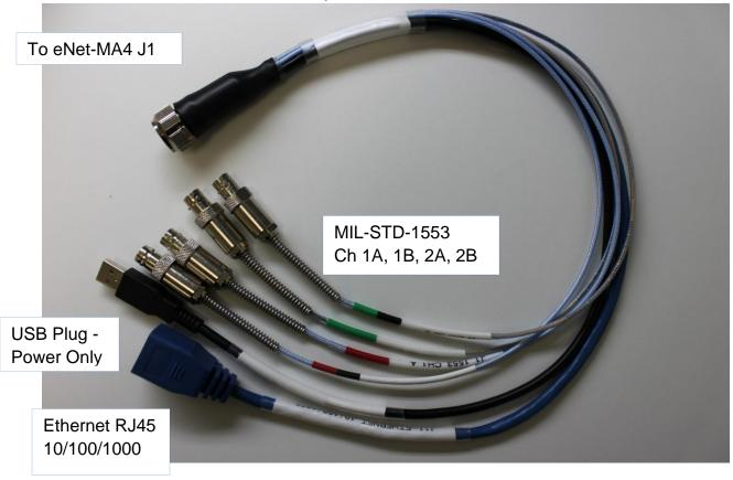
Figure A-1: Optional ENETCAB-1553-J1-02 Cable Assembly
