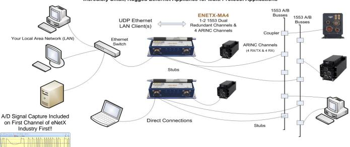
**eNetX-MA4**<sup>™</sup> is an innovative product for "remoting" 1553 & ARINC-429/717 operations on 10/100/1000 Ethernet local area networks (LAN). eNetX-MA4 is a very small, low-power, rugged device that provides real-time UDP connectivity to for 1-2 dual redundant 1553 (A/B) busses and 4 ARINC channels. Tested to MIL-STD-704F/810G/461F and DO160.
