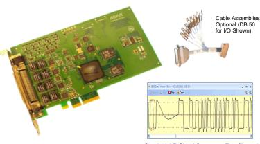
Standard A/D Signal Capture on First Channel
