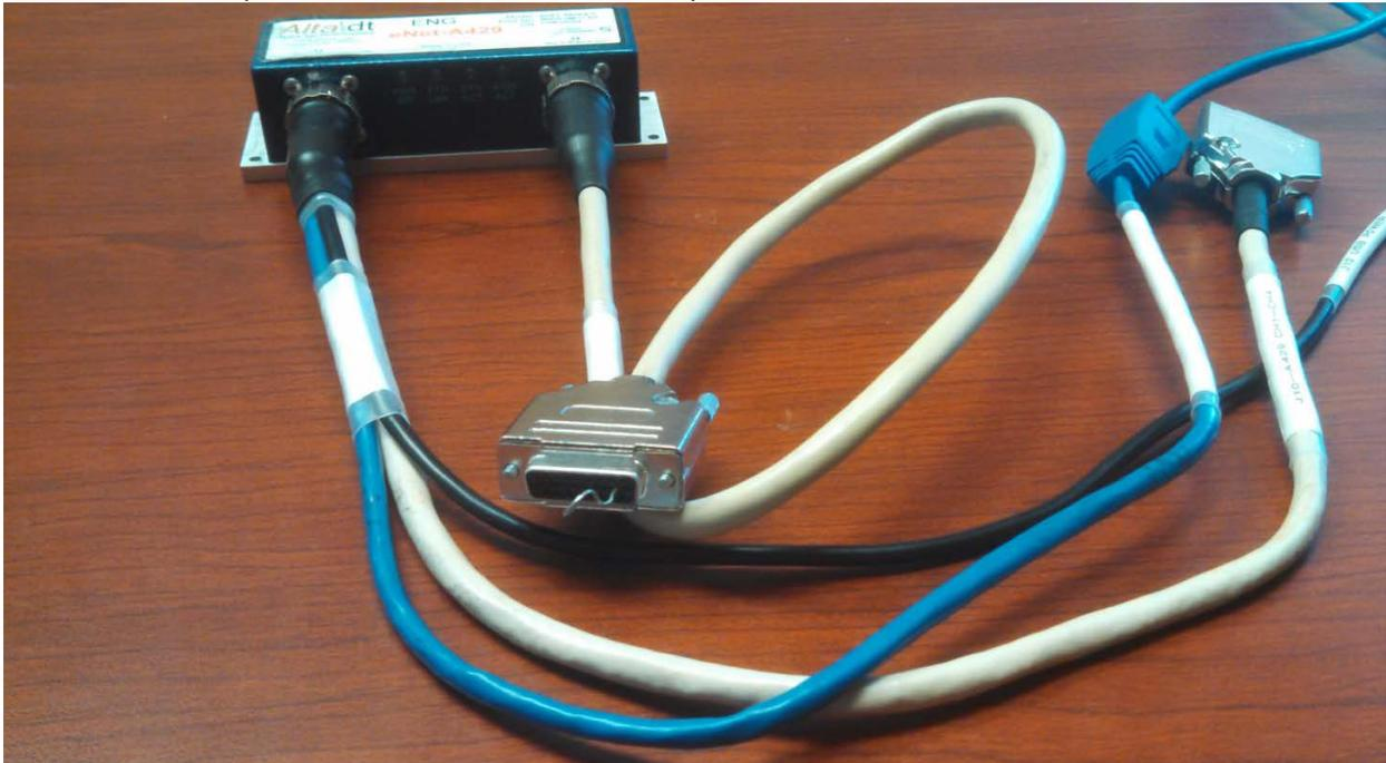
Disconnect power to the ENET-A429, jumper pin 23 to GND, then apply power to the ENET-A429.
