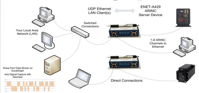
**eNet-A429**™ is an innovative product that provides "remoting" of ARINC operations on 10/100/1000 Ethernet IP/UDP local area networks (LAN). eNet-429 is a small, low-power, rugged device that provides connectivity for 1-8 ARINC 429/575/573/717 Channels - Ideal for remoting ARINC connections for in-field applications or point-point lab usage.
