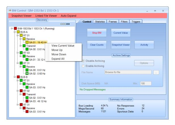
At the SA level, you can also select "View Current Value" to see the most recent message for that SA. This is identical to clicking the "Current Value" button in the "Control" tab. If you double-click on an SA node this will bring up the "Current Value" viewer for that SA.
