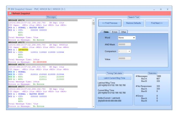
A menu-strip provides the option to "Refresh Snapshot" – Will update the display with the current messages in the BM Snapshot Buffer (up to 1000 messages). These are the most recent messages seen by the BM. The messages are displayed on the left in a scrollable window.
