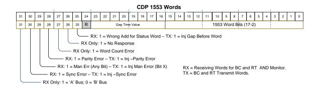
The upper 16-bits provide information on which bus the word was on, any errors on the word and the dead-bus gap time (100ns LSB) from the previous word. The lower 16-bits contains the actual 1553 word (CMD, STS, or DATA).
