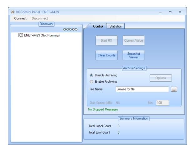
The menu-strip provides options to **Connect** and **Disconnect** to the ENET APMP device. You must connect to a device to enable the "Start RX" button.
