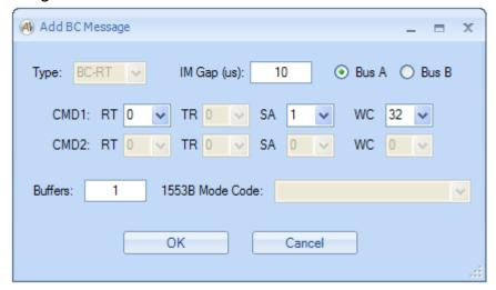
Appropriate fields are enabled or disabled based on the selected message type (BC-RT, RT-BC, RT-RT, or MODE). For MODE messages, a combo-box is provided to select standard 1553B mode codes. You can set the inter-message gap (time from the end of the previous message to the start of this message). You can select the bus for the message (bus A or bus B). You can also specify the number of BC buffers to allocate for the message.
