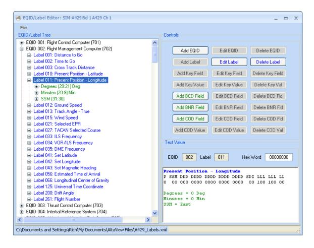
The editor shows the defined EQID and labels in a tree on the left and provides controls on the right. If a Label node is selected in the tree, the "Test Value" panel is enabled – you can enter a value in the "Hex Word" box (then click in the rich-text box below it to update the value) and this will display the interpreted label value. Controls are enabled based on the selected level in the tree.
