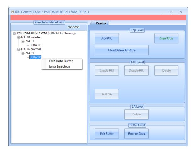
Right-clicking on a Buffer node will give you the options "Edit Data Buffer" and "Error Injection". Double-clicking on a Buffer node will open the "Edit Data Buffer" dialog for that buffer.
