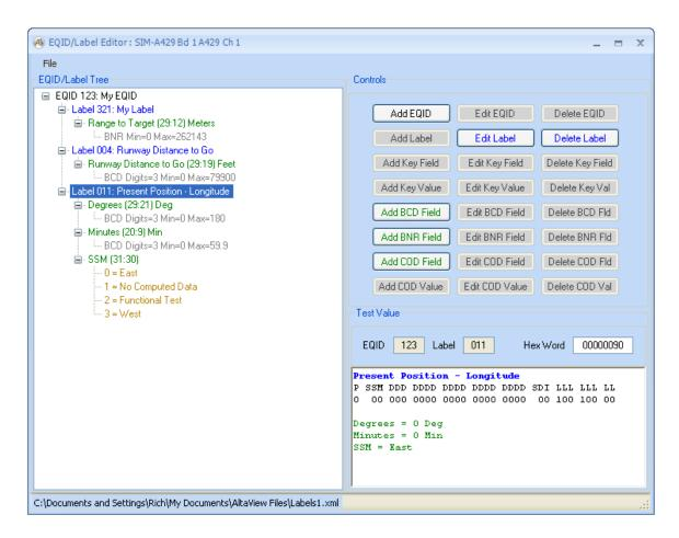
The "Key Field" is used when one field of bits in the Label determine how the rest of the word should be interpreted. For example, Label 037 "HF COM Frequency" uses bit 9 as the "Word Identifier".
