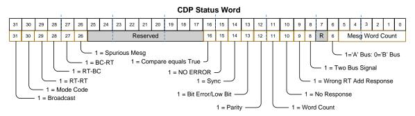
This word provides information on the message type in bits 26-31, message-level error information in bits 8-15, the bus the message occurred on in bit 6, and the count of DATA words in the message in bits 0-5.
