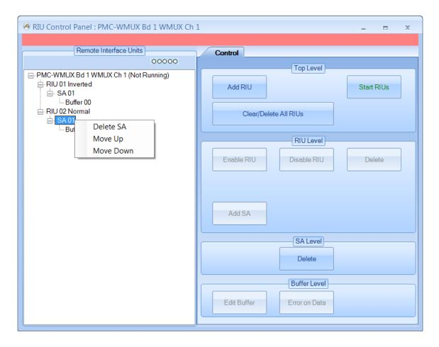
Right-clicking on a SA node will give you the options "Delete SA", "Move Up", and "Move Down". "Delete SA" removes the SA from the tree and frees all resources associated with the SA. The "Move Up" and "Move Down" options allow you to reorder the SA nodes in the tree.
