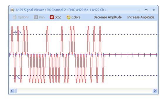
This shows a high-speed (100 KHz bit rate) A429 signal.
