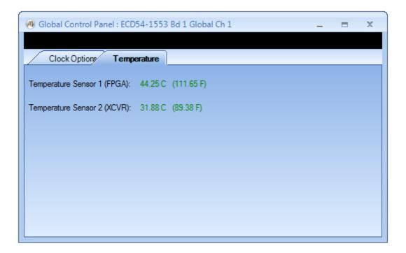
The temperature sensors have a range of -128 to +128 degrees Celsius (in steps of 0.125 degrees Celsius). Temperatures from 0 to 50 degrees Celsius are displayed in green. Temperatures above 50 degrees Celsius are displayed in red. Temperatures below 0 degrees Celsius are displayed in blue.
