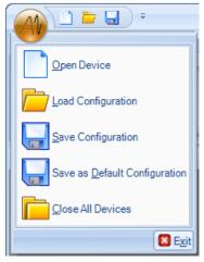
You can save configurations to files other than "AV\_Default.xml" using the "Save Configuration" option under the Logo-Button menu – this allows you to specify the filename for your configuration file.
