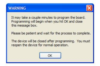
DO NOT INTERRUPT THE PROGRAMMING PROCESS. If this process is interrupted the firmware load will fail and the board will have to be returned to Alta to be reconfigured.
