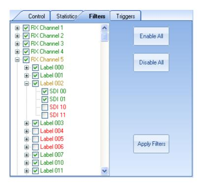
The "Enable All" button will enable the MCRX to capture all messages on all RX channels. The "Disable All" button will block all messages. The "Apply Filters" button will apply the selected filter settings. No changes take effect until the "Apply Filters" button is clicked.
