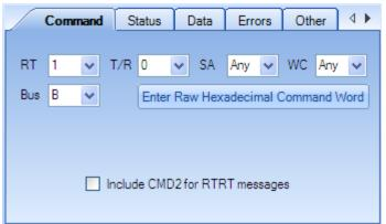
Under the "Command" tab, we would select Bus B, RT 1, and T/R of 0 (receive).
