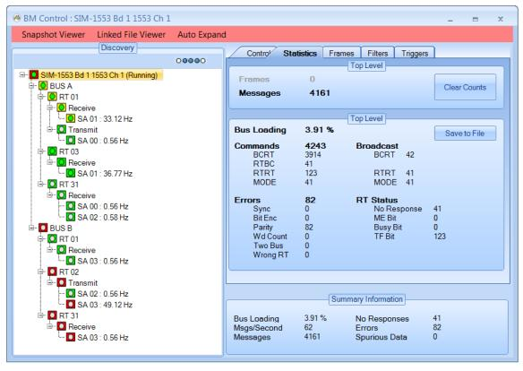
The upper panel provides a top-level count of Frames and Messages. Frame counts are only enabled if a start-of-frame message has been defined in the "Frames" tab. A "Clear Counts" button is provided here as well – this is identical to the "Clear Counts" button on the "Control" tab.
