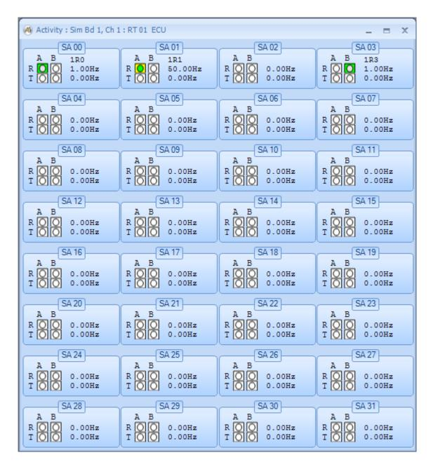
As for the RT level, four activity icons show activity by Receive and Transmit on Bus A and Bus B for each SA. On the right, the current message frequency is displayed for both receive and transmit messages. If you left-click on one of the SA panels the view will switch back to the RT level.
