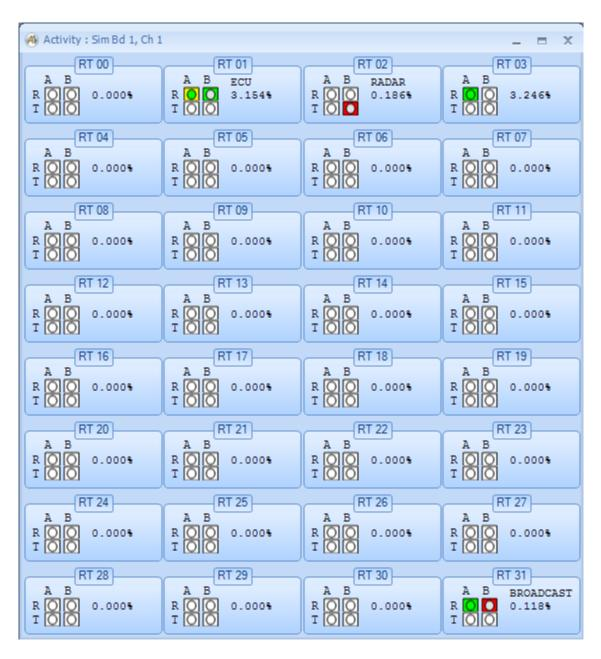
For any given RT address, four activity icons show activity by Receive and Transmit on Bus A and Bus B. The percentage bus loading is also shown for each RT. If you left-click on one of the RT panels, the view changes to show activity for all Sub-Addresses (0-31) for that RT address.
