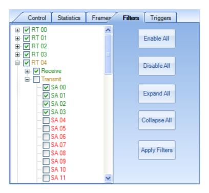
The "Enable All" button will enable the BM to capture all messages. The "Disable All" button will block all messages. The "Expand All" button will expand all nodes
