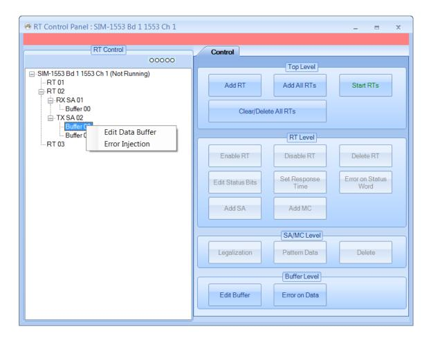
Right-clicking on a Buffer node will give you the options "Edit Data Buffer" and "Error Injection". Note that the "Error Injection" option is only provided for Transmit buffers. Double-clicking on a Buffer node will open the "Edit Data Buffer" dialog for that buffer.
