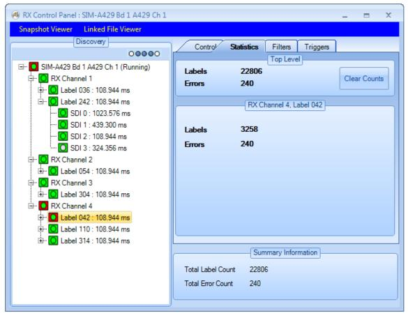
The upper panel provides a top-level count of labels and errors. A "Clear Counts" button is provided here as well – this is identical to the "Clear Counts" button on the "Control" tab.
