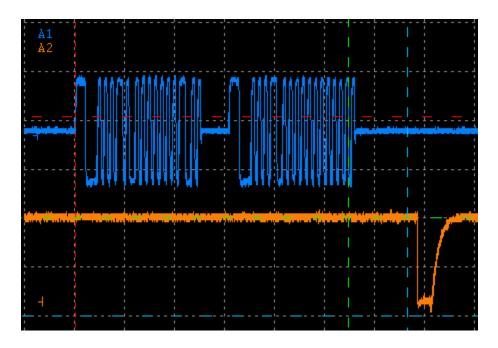
Even though our trigger is looking for the Command word, the entire message must complete before the trigger signal is generated. In this case the trigger signal is seen approximately 10 microseconds after the end of the Status word from the Remote Terminal.
